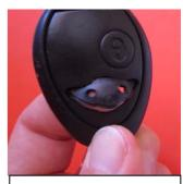
4. Push out **back mounting plate** from top shell to make room for new button.
