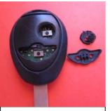
6. When **both buttons are removed,** remote is ready for fitting our silicone button in.
