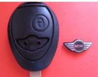
3. Remove **Silver Wing** (if still attached to back mounting plate), by peeling it off.
