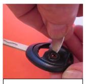
5. Once wing button is removed, carefully **cut out round button** using Stanley knife or scalpel.
