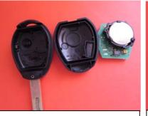
2. **Separate** electronic parts from plastic shell. Do not remove battery.
